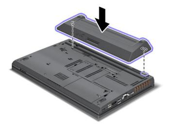
4. Slide the battery latch to the locked position.
